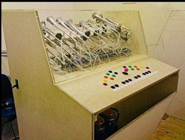
The Klaxophone's "Doncamatic" like car horns
